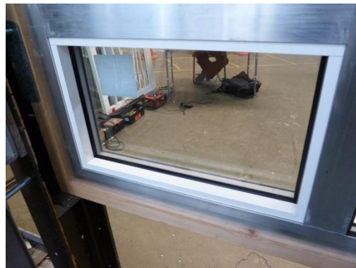
Figure 11 Internally glazed light viewed from non-attack side
