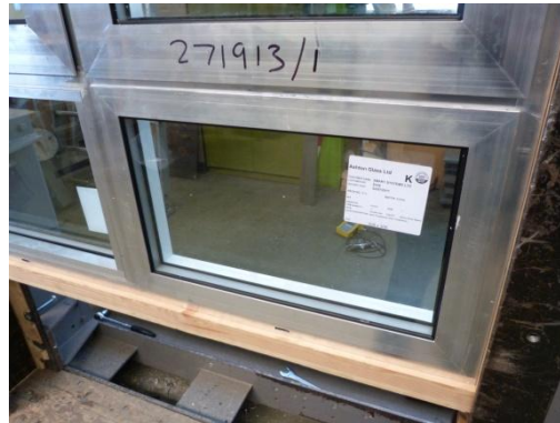
Figure 9 Internally glazed light viewed from attack side
