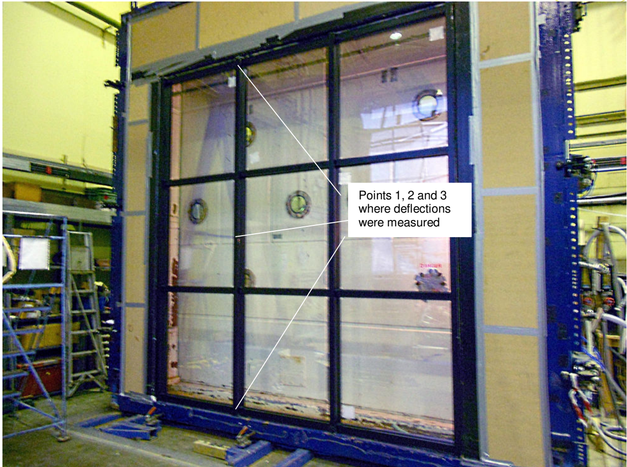
Figure A3. The test specimen showing points 1, 2 and 3 where deflections were measured.
