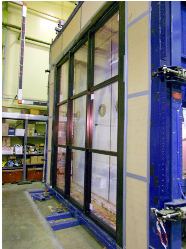
Figure A2. The test specimen installed in the BRE 'B' Weathertightness test rig
